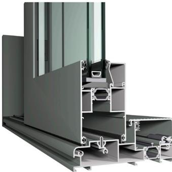
**MONORAIL.** A Monorail combines a movable vent on one side of the frame with a stationary glazed element anchored directly into the frame on the other, creating a minimalistic look. Utilizing a fixed panel in lieu of fixed vent reduces sight-lines while allowing for the integration of optional inward opening window(s) into the interior side of the frame. However, it is possible to mount the fixed portion on the outside, when glazing the unit from the exterior is desired.
